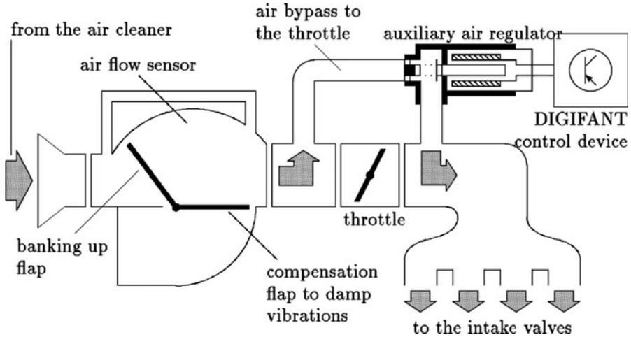
Fig. 16.3 Principle of the engine idle speed control
