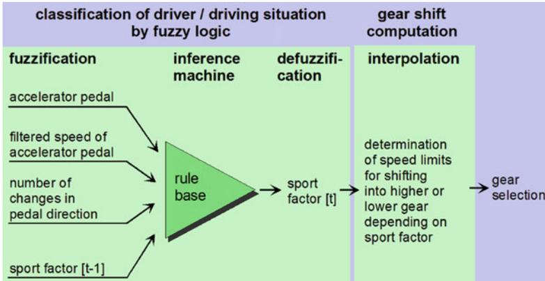
Fig. 16.9 Flowing shift-point determination with fuzzy logic
